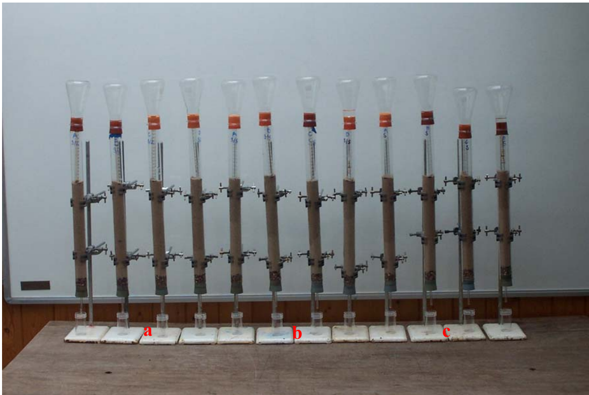
Figure 14: 12 eluting soil columns, 4 containing a zeolite amendment rootzone (a), 4 containing another zeolite amendment rootzone (b), both incorporated at a ratio of 90:10 (sand:zeolite v/v), and 4 control columns contain 100% sand (c).
