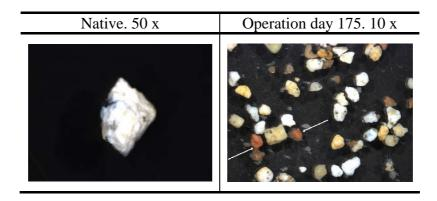
**Figure 6.** Stereomicroscopic observation of a native zeolite particle and zeolite particles after 150 days inside the reactor SBRZ.
