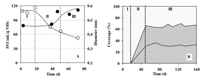
**Figure 4.** A) Sludge volumetric index (SVI) ( $\bigcirc$ ) and average feret diameter ( $\bullet$ ). B) Percentages of zeolite fully covered  $\square$ , partially covered  $\square$  and no covered  $\square$ .
