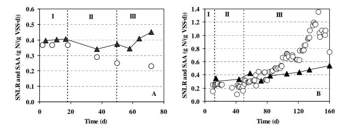
**Figure 1.** Specific Nitrogen Loading Rate (SNLR) applied ( $\bigcirc$ ) and Specific Anammox Activity of the biomass (SAA) ( $\triangle$ ) in reactors SBR1 A) and SBRZ B).
