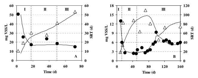
**Figure 3.** Biomass concentration in the effluent (mg VSS/L) ( $\bullet$ ) and sludge retention time (SRT, d) ( $\Delta$ ) in reactors SBR1 A) and SBRZ B).
